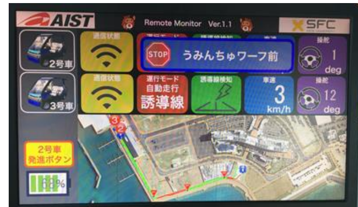
Remote monitoring / control monitor screen
