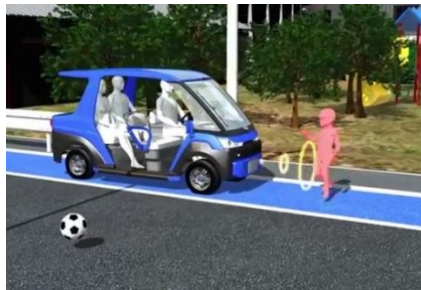
Obstacle detection and safe stop
